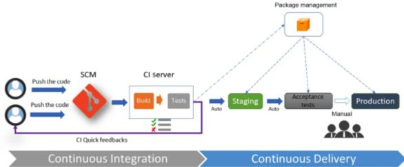
The preceding diagram shows that the CD process is a continuation of the CI process. It represents the chain of CD steps, which are automatic for staging environments but manual for production deployments. The package is generated by CI and stored in a package manager, and that it is the same package that is deployed in different environments.
